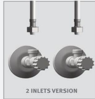
**MAKE SURE THAT THE FILTERS ARE INSTALLED BETWEEN THE FLEXIBLE PIPE AND THE SHUT OFF VALVE/ANGLE VALVE (NOT SUPPLIED).**
